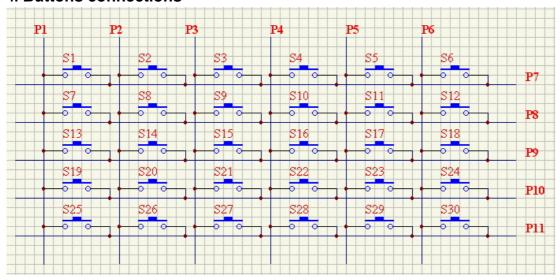
Connect 30 buttons for playing 30 different mp3 files in the SD card .
