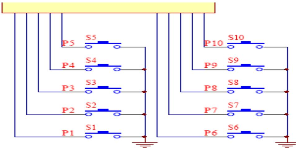
Connect 10 buttons for playing 10 different mp3 files in the SD card .
